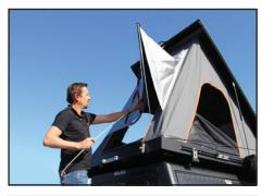
**Step 7**: Place pole into lower tube and then hook onto canvas eyelet.
