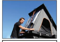
**Step 3**: After you've lifted the lid a little, the gas struts will kick into action and open the tent fully.
