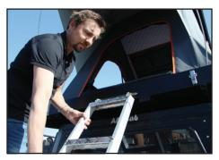
**Step 9 :** Slot ladder onto catch and secure. Note, additional ladder brackets can be specified (or ordered) and installed on the sides for side entry.
