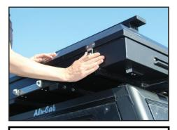
Step 13 :Secure lid by fastening both catches.
