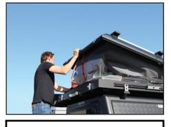
**Step 12**: Grab handle on roof when it comes into reach, and use it to pull the lid closed. Make sure the canvas is tucked in on both sides before closing. Also, make sure at least one window is open when closing tent or the trapped air makes closing very difficult.
