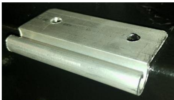
Figure 6: C-Clamp extrusion with holes drilled into vehicle
