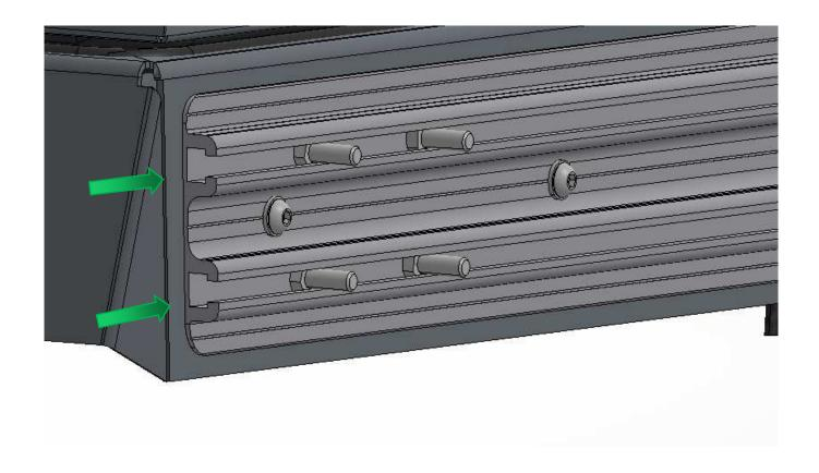
Position the rear bracket over the bolts you placed in the extrusion slots. Fasten the bracket to the extrusion using the supplied nuts and washers.
