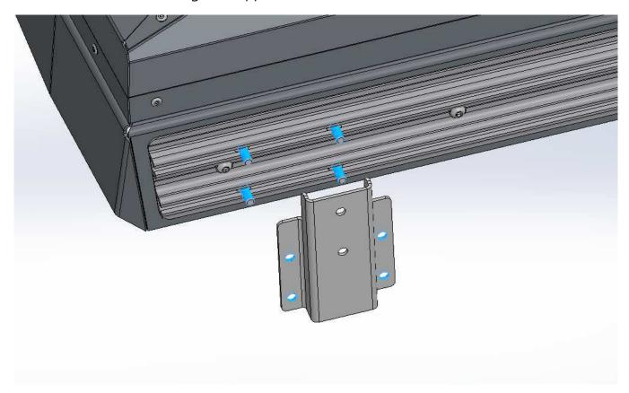
When fastening the front bracket, do not tighten the bolts to fix the bracket in place. Allow for the bracket to be able to shift/slide along the extrusion so the bracket can be aligned with the correct mounting holes on the awning.
