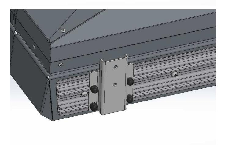
Mount the awning to the brackets, starting from the rear, using the button head bolts and M8 oversized washers.
