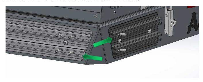
Slide 4 M8x20 hex head bolts into the extrusion slots at the front side end of the roof conversion.
