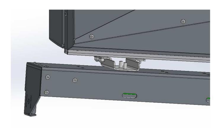
Once the correct positioning for the front bracket is found, remove the awning and tighten the bolts attaching the brackets to the roof conversion and place the black nut-caps on the nuts.
