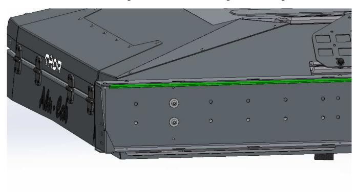
Fit the black nut-caps on the nuts at the back of the bracket to complete the fitment of the awning to the roof conversion.
