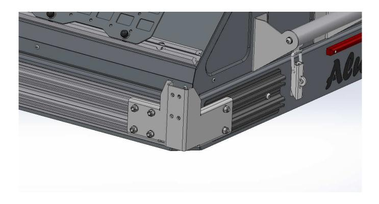
Position the front bracket over the bolts you placed in the front extrusion slots. Fasten the bracket to the extrusion using the supplied nuts and washers.
