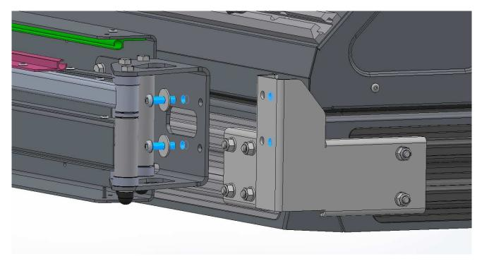
Align the front bracket mounting holes with the 2nd set of mounting holes on the channel of the awning. Insert the two button head bolts to check the for the correct positioning.
