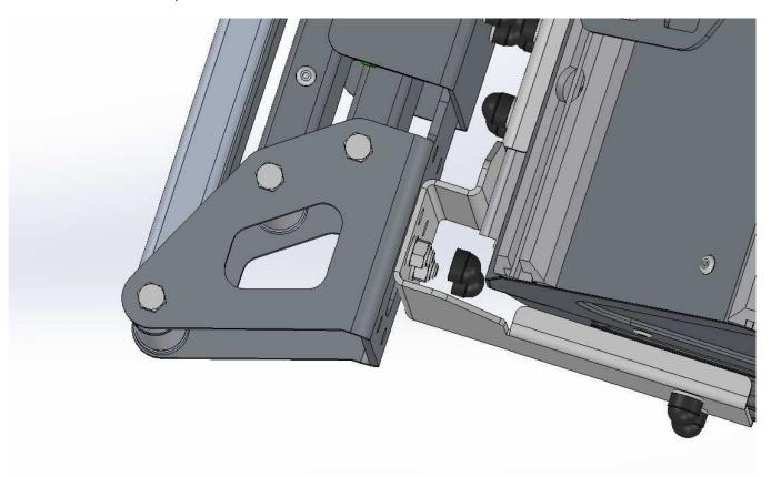
Fasten the front end of the awning to the front bracket using the remaining fasteners.
