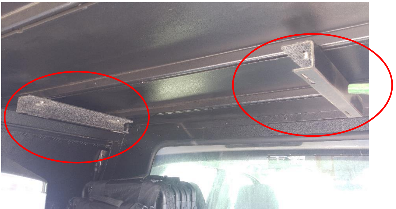
Figure 3: Table brackets installed
