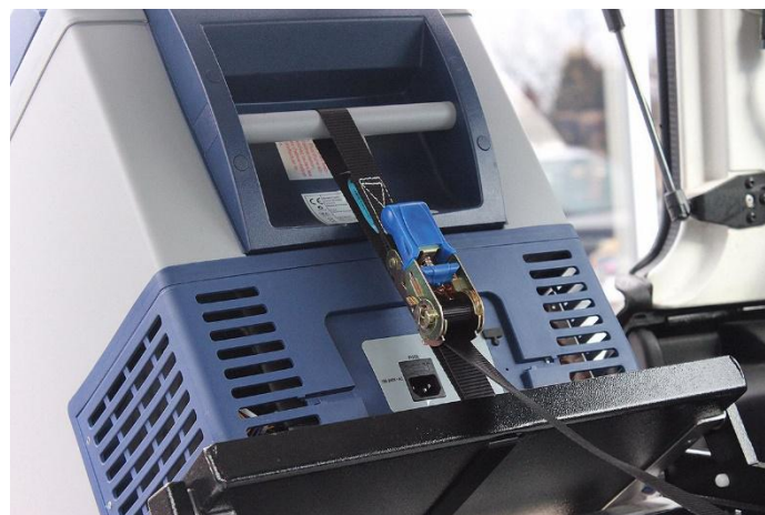
Figure 6: Ratchet strapped fridge.
