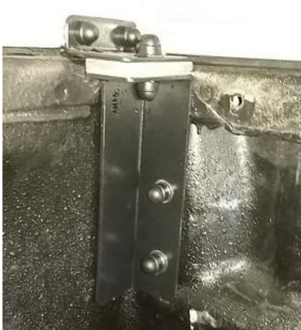
Figure 16: Front Support Bracket Installed
