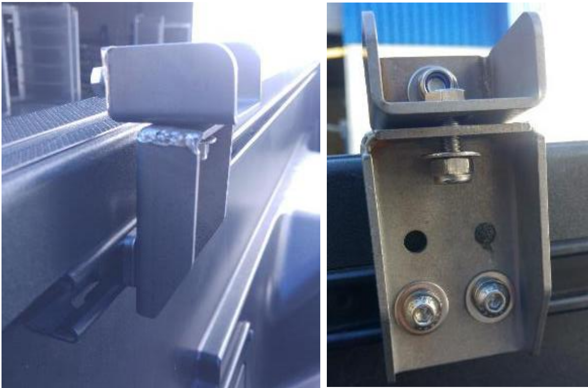
Fig 15: Photos of Bracket kit assembled in Tacoma Load Bin
