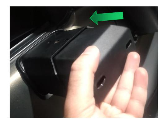
Lock the Inner Part in place by fastening with the supplied M6x20mm Button Head bolts, Spring Washers and Large flange washers, in 3 places (1 combination on top and 2 combinations at the bottom of the extension unit) as per images below
